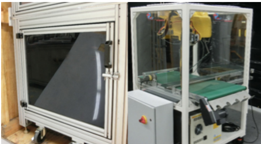
Figure 2. A comparison of a machine built using an aluminum frame (right) versus a machine using a steel base (left).
